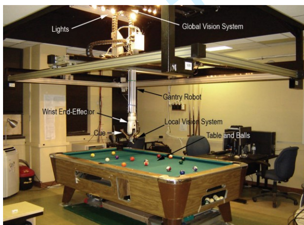
Fig. 1. Gantry-based pool playing system [2]
