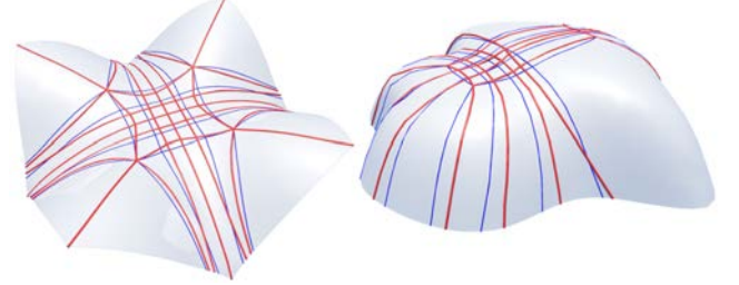
Figure 11: Rib network before (blue) and after (red) rib flow optimization for Guscio (left) and Botanic (right).
