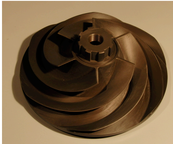
Figure 6. The six-bladed centrifugal impeller of the VAMPIRE turbopump.
