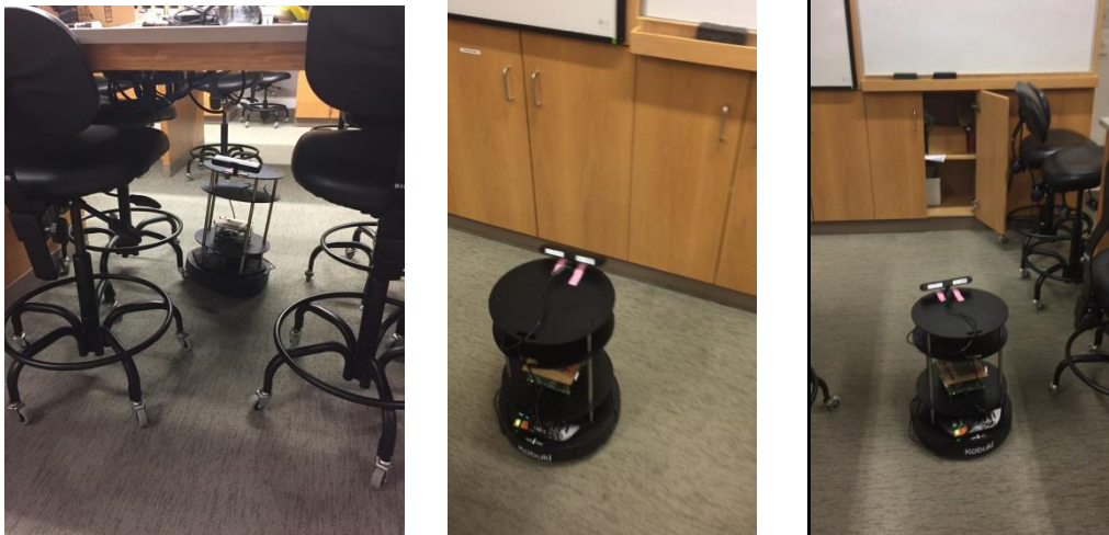
Figure 25. The two scenarios on the left were omitted from training. We can see that after some training, the robot managed to decide to go under the table in between the chairs. Hence, care was taken to put chairs closer together in the future to address the first scenario. The third scenario includes an open cabinet to address the second scenario.
