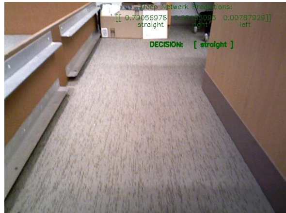
Figure 50. A sampling of scenarios where the neural network made live decisions and the probabilities of each possible decision. Large images are shown for the second half of the examples in order to make the numbers easier to see.
