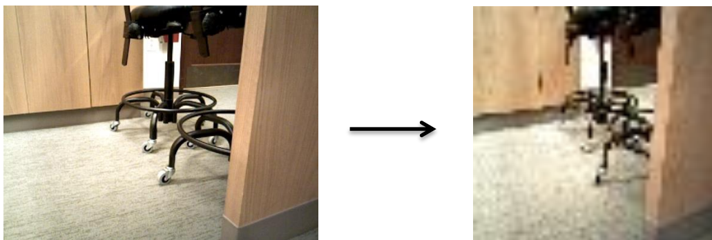
Figure 45. Image provided to network to demonstrate activation values. Recall that the network takes 64 x 64 images. An enlarged version of the downsampled image is shown.
