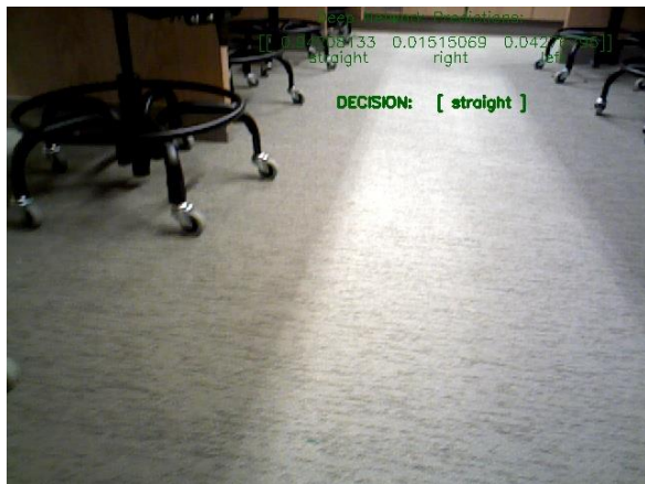
Figure 50. A sampling of scenarios where the neural network made live decisions and the probabilities of each possible decision. Large images are shown for the second half of the examples in order to make the numbers easier to see.
