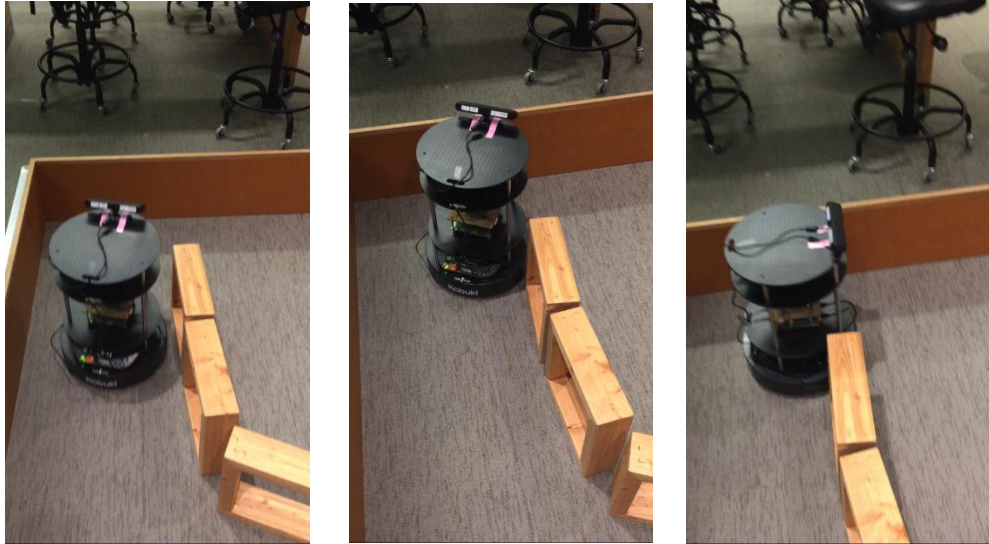
Figure 39. Scenario: new environment; obstacle avoidance with wooden blocks
