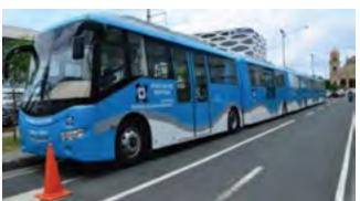
A hybrid road train that runs on diesel and electric power is being developed by the Perlas government. The prototype can carry 260 passengers.
