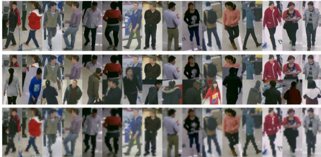
Figure 4. First row original RAP dataset. Second row occlusion RAP dataset where the images have been occluded from 50 to 80% by pasting the upper body of another subject. Third row low resolution RAP where the image are downsamples of a factor 4 on width and height respectively.
