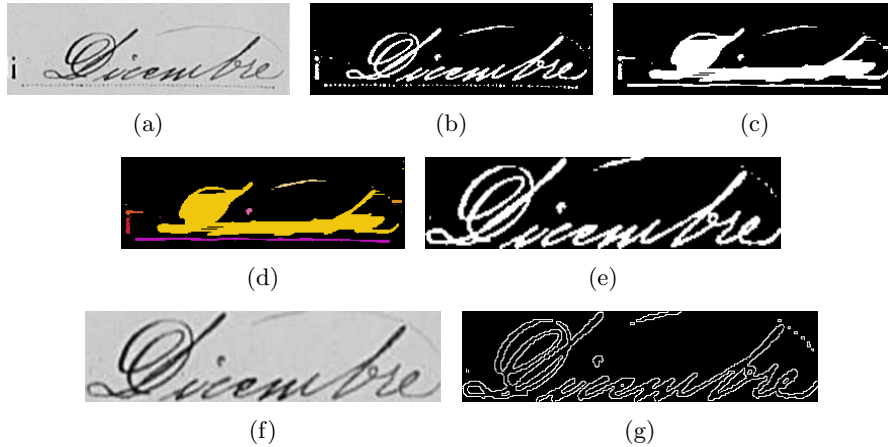
Fig. 1: Example of pre-processing steps applied to an handwritten word image. (a) is the raw input grayscale word image, (b) the result after binarization process, (c) the graphical output of the RLSA algorithm. Connected components are then labeled (d) and the bounding box of the biggest component is extracted (e) and (f). In (g) is reported the output of Canny algorithm applied on (e).
