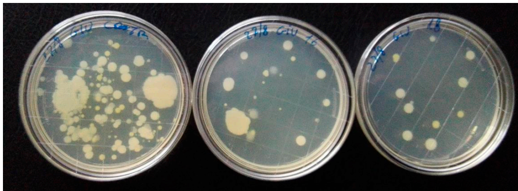
Figure 2. On the left, Petri dish showing baseline volunteer contamination after auscultation. The other two plates show the reduction of the contamination after one cycle (5 min) of UVC disinfection obtained by LED 16 (center plate) and LED 18 (plate on the right). Irradiation was performed after 1668 cycles of LEDs functioning.
