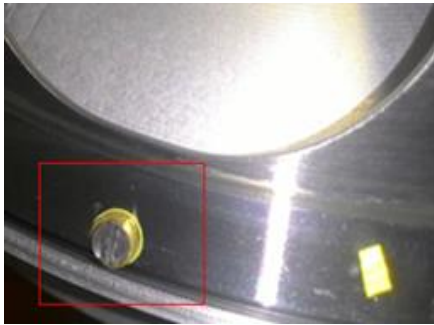
Figure 2. The mechanical method of the flywheel balancing.
