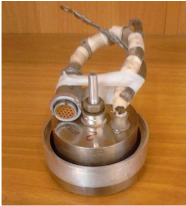
Fig. 1. Electro motor DBE63.
