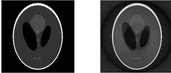
Fig. 5. Original image on the left and reconstructed image on the right with the intensity artefact.
