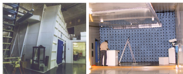
Fig. 1. Outer view and inner view of the GTEM 3750.
