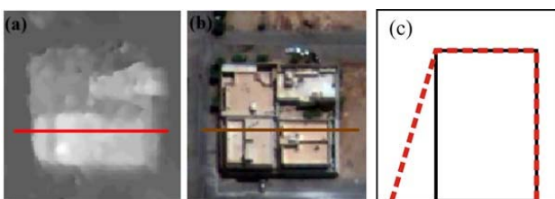
Figure 3. (a) Sample DSM of image matching, (b) corresponding image with cross section line, (c) schematic cross section from the side (red: DSM, black: original object)
