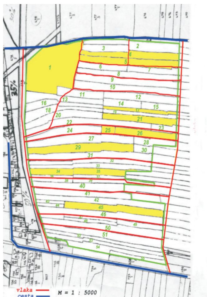
Fig. 1: Arrangement of plots on research object (yellow labelled lots are lots selected by sampling, red - skidding trail, blue - forest road)
