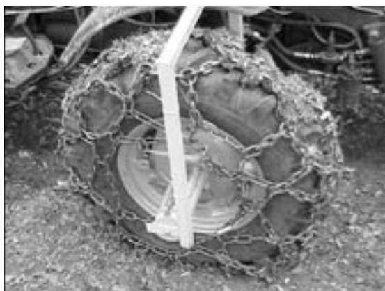
Figure 3: Chains on a powered tractor wheel
