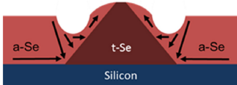
Figure 35. Model of change in morphology under the focused laser spot for saturated growth of PC in an a-Se film on a rigid Si substrate. A boundary through forms due to the density increase in t-Se.
