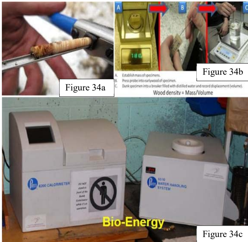
Figure 35. Example of wood properties testing procedures and equipment. Figure 34a. shows the removal of wood from an increment borer. Figure 34b shows the weighing and dunking of wood samples to determine density, and Figure 34c shows the bomb calorimeter where thermal potential is measured.
