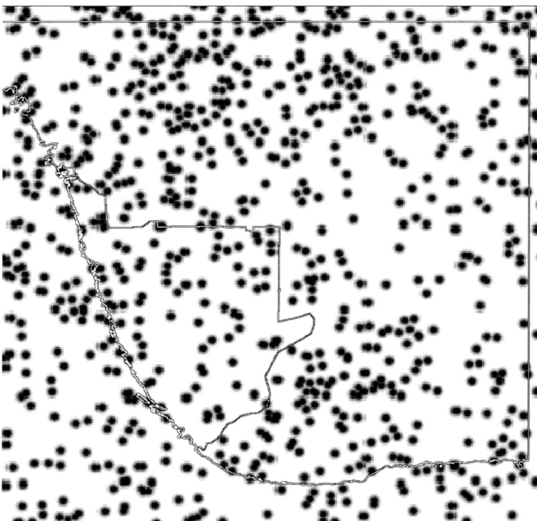
Figure 11 - Probability density map of positive polarity lightning strikes. The values in the map represent the relative likelihood of a strike having happening in that area in the study period. Increasing probability is indicated by an increased intensity of black.
