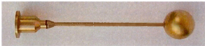
Figure 2.12: An example of a Langmuir probe to measure ion density
