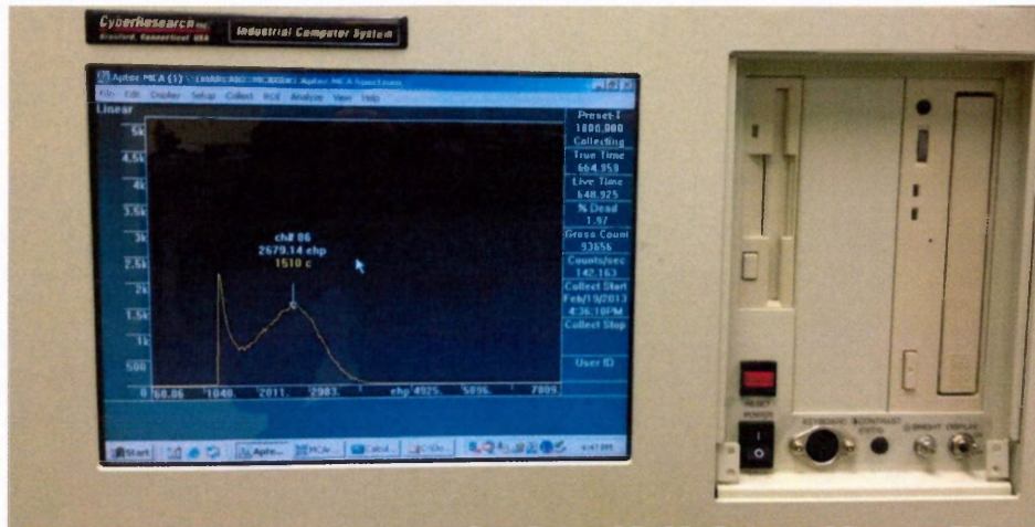
Figure 3.5 The computer is equipped with MCA card and software for analysis and data output. For each PHS experiment, the spectrum can be viewed in real-time which is shown here on the screen.
