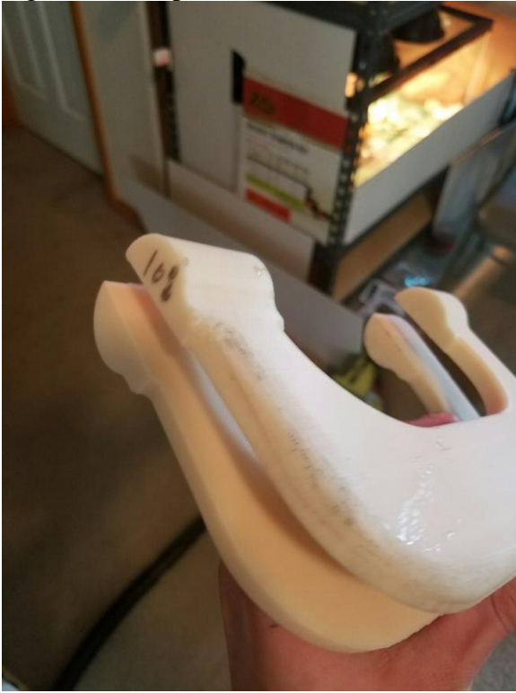
Figure 14 – Imprint #1 Design 2.0 Test Print Success
