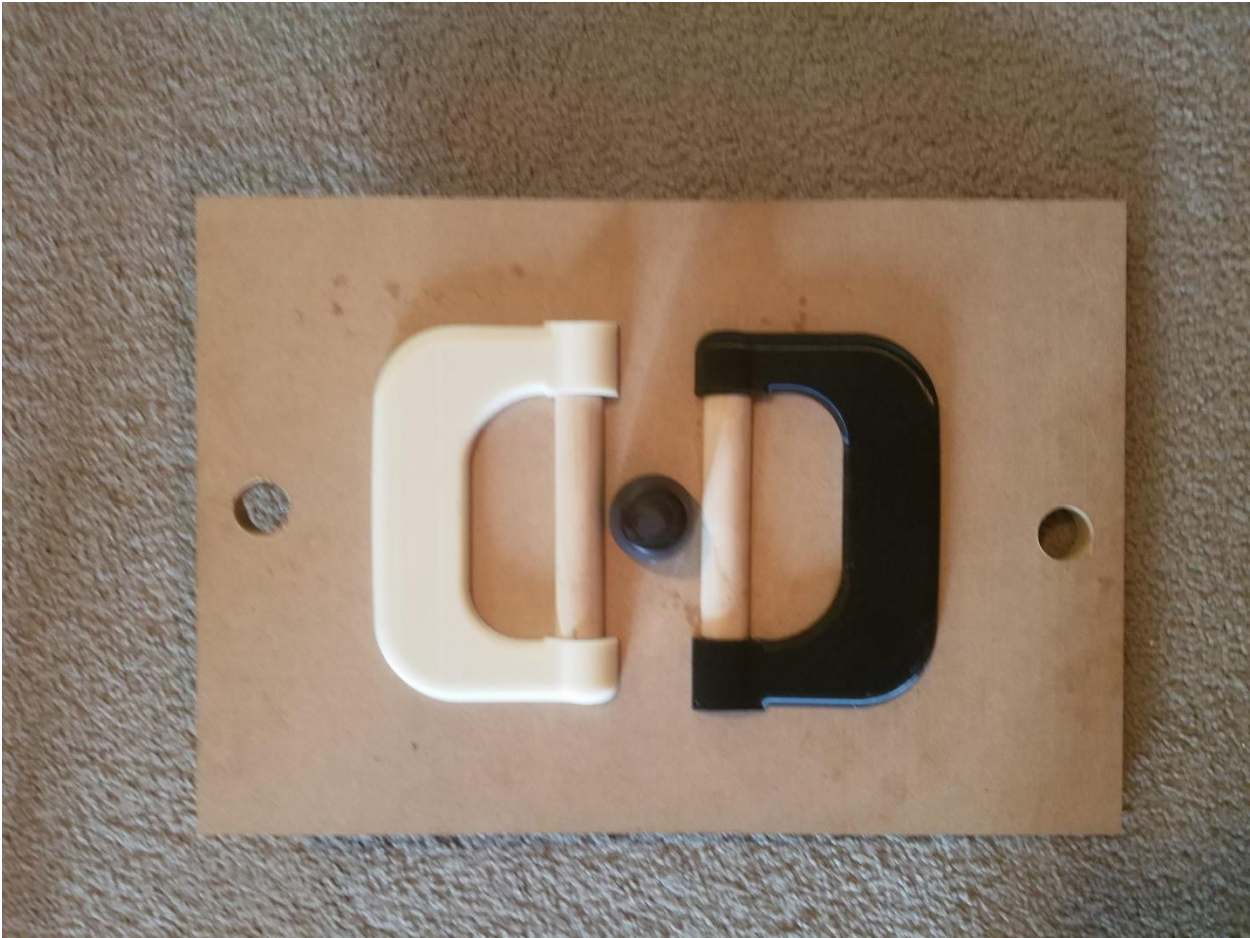
Figure 17 – Matchplate Drag(Top) Assembly
