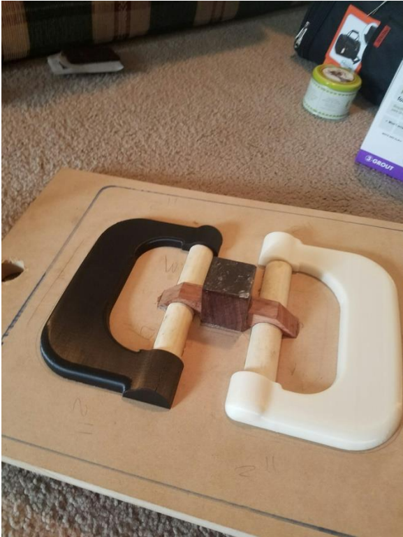
Figure 16 – Matchplate Cope(Bottom) Assembly
