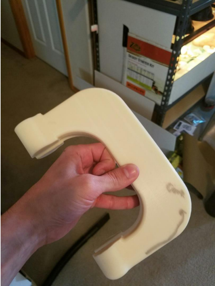
Figure 12 – Imprint 2.0 Test Print: Error Recorded, Failed to print continued drafted edge of Fillet
