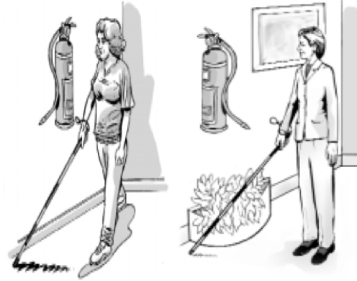
Figure 6. Wall mounted cane hazard made safe.
