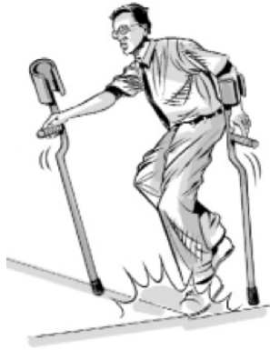
Figure 4. Tripping hazard of uneven path of travel.
