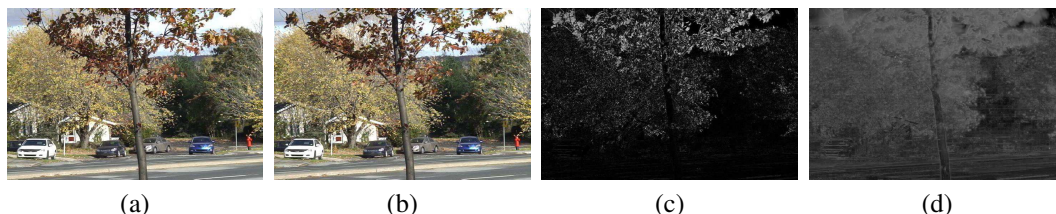
Figure 5.2 – Sequence fall of "background motion" category: (a) result of Photomontage ; (b) GT image; (c) absolute gray-level difference of (a) and (b); (d) negative log likelihood map of (b) as compared to the GT model. Although visually identical to the GT image, the result achieves very poor image metrics scores (AGE: 23.9, pEPs: 0.32, pCEPs: 0.11, MS-SSIM: 0.73, PSNR: 15.6, CQM: 16.7), due to tree branches not perfectly aligned, but average probabilistic metric value (PM: 9.707).
