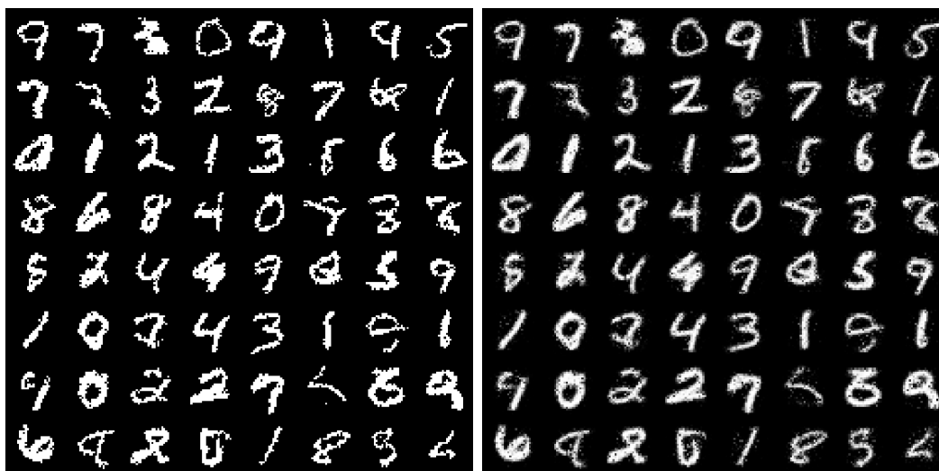
Figure 4.7: Left: samples from ConvNADE+DeepNADE trained on binarized MNIST. Right: probabilities from which each pixel was sampled. Ancestral sampling was used with a different random ordering for each sample.
