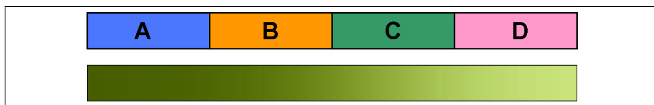
Figure 1.1 Top: Discontinuous gradient where A, B, C, and D represent different materials connected in series. Bottom: Continuous gradient in which the surface chemistry is varied from a high degree of functionality (left) to a low degree of functionality (right).
