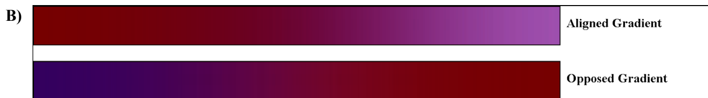
Figure 1.9 A) Schematic illustrating controlled-rate infusion. After infusion, the bottom of the substrate has been soaking for a longer period of time and, therefore, has a higher degree of functionality, whereas the top has been soaking for a shorter period of time and, therefore, has a lower degree of functionality. B) Schematic of aligned (top) and opposed (bottom) gradients.
