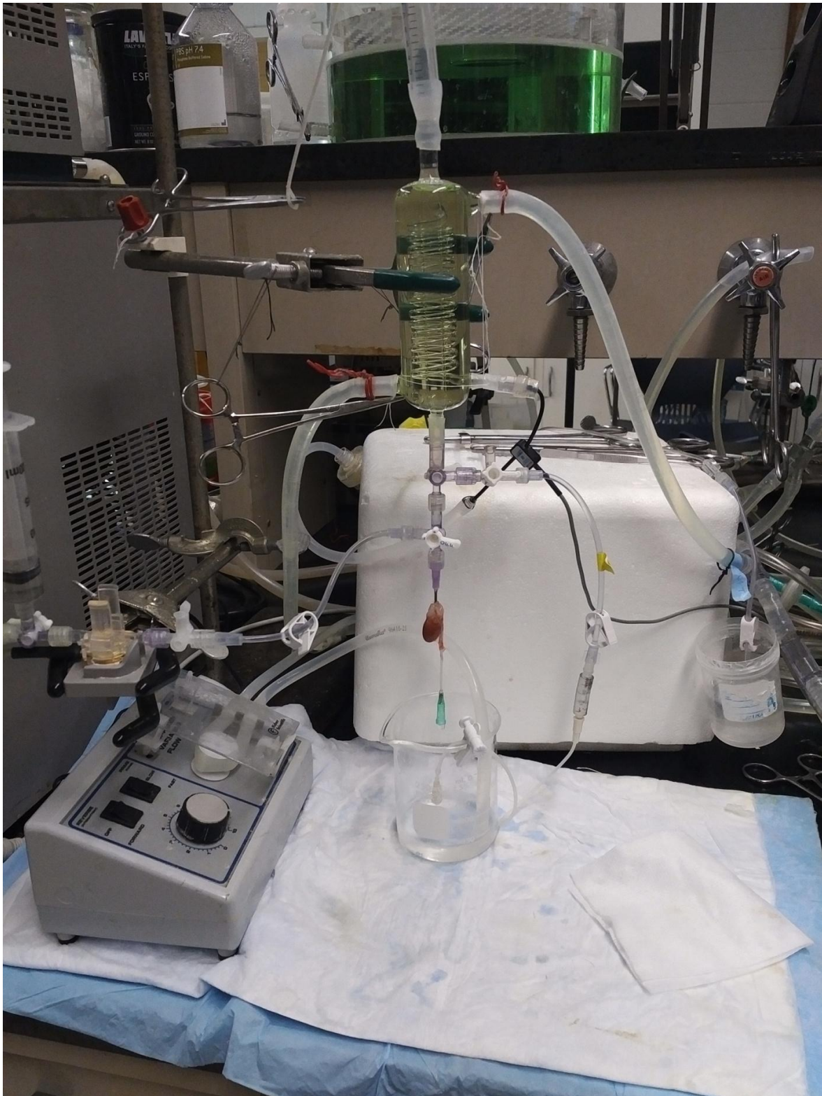
Figure 2 shows the entire system assembled and running. The green color in the glassware is from the circulating coolant. The beaker beneath the heart is a reservoir for the circulating MPS. The particulate filter and oxygen membrane are present, but not visible in this photo.
