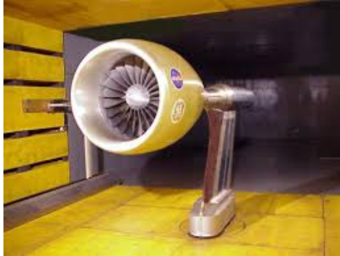
Figure 3.1 SDT2-R4 installed in wind tunnel.
