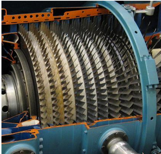
(a) Several rows in an axial flow compressor.
