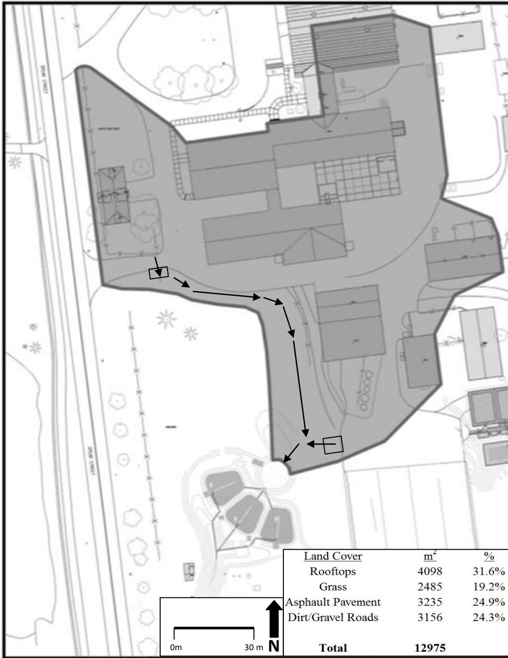
Figure 1 – Watershed drainage area of MRC Bioretention Cells. Runoff from the southwest (institutional) and southeast (agricultural production facility) ends of the complex is channeled into the forebay of the bioretention cells via two grass lined swales (the location and direction of flow is conceptually depicted by arrows). The four main land cover classifications of this watershed are described in text, along with their area and percent of total watershed.
