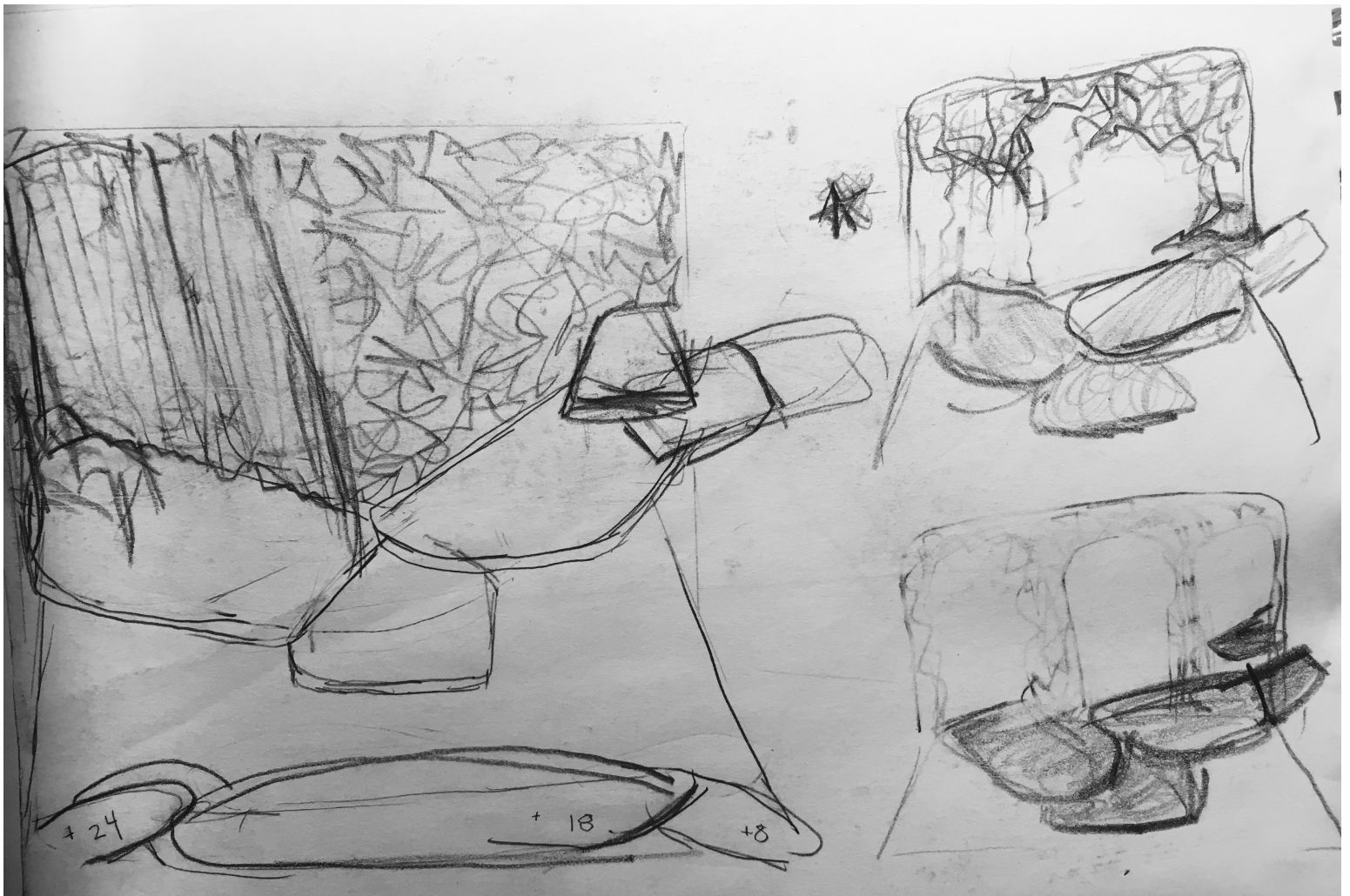
Figure 10: The first complete design proposed to the director, technical director, and thesis supervisor. Eight platforms stacked to form Lucy's bedroom, Lucy's tomb, Dracula's castle, the asylum, and a rake platform leading to Renfield's cell. With the final decent into Dracula's tomb, these platforms were to pivot upstage to reveal an open trap.
