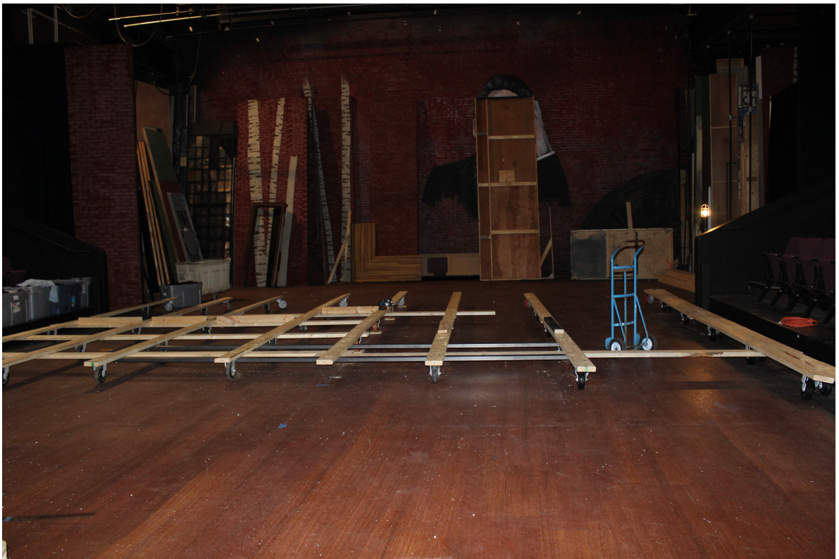
Figure 22: Carriage Allowing for Upstage and Downstage Movement of Set
