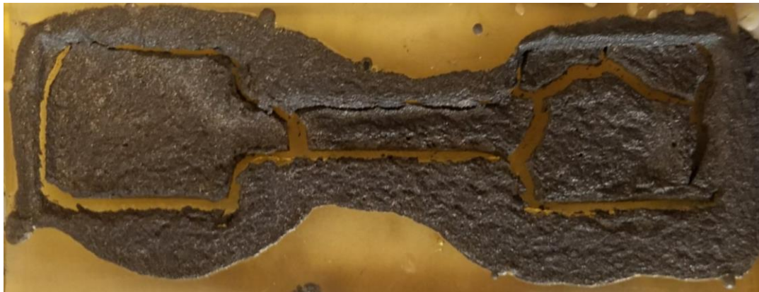
Figure 19: 25 vol.% Ni tensile specimen attempt cracked and fell apart in the mold while drying.
