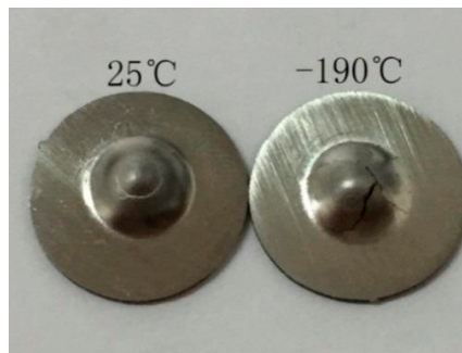
Figure 3. Macrophotograph of the fracture sample at 25 °C and −190 °C.
