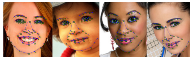
Fig. 4: Special points that Luxand uses for face recognition.
