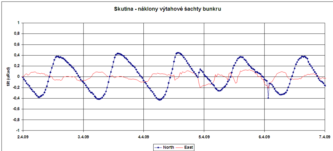
Fig. 5 The development of the tilt of Skutina fortress in April 2009
