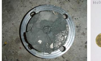
**Fig. 9.** Horizontal-vertical crack rock sample from the borehole H III after test of fracturing
