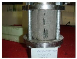
**Fig. 8.** Rock sample cored in H 111 after the laboratory fracturing experiment – on the front face of the sample is apparent vertical fracture
