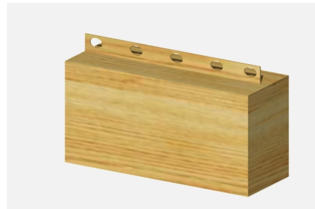
Figure 3: Production of samples. The wooden part of the profile with the encompassed mesh.
