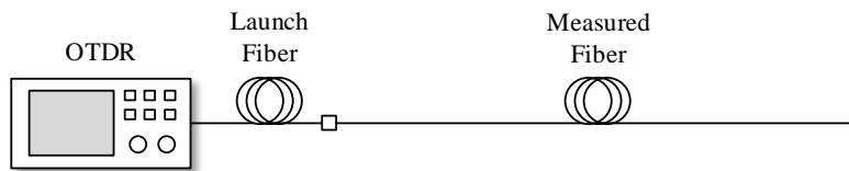
Figure 44: Topology for OTDR measurement
