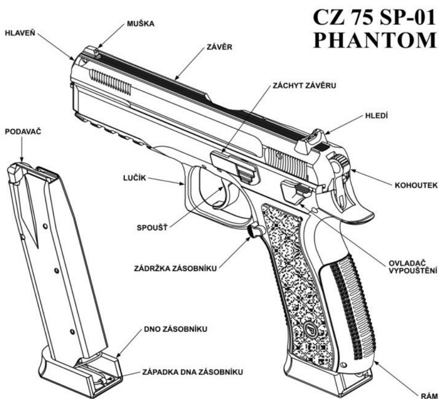
Obr. 2.1 Popis pistole CZ 57 SP-01 PHANTOM [2]
