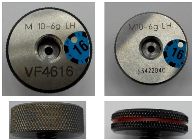
Figure 26: Good and faulty reference thread gages
