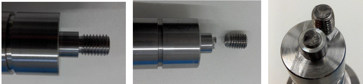
Figure 17: Examples of good and fractured shaft (other parts removed)
