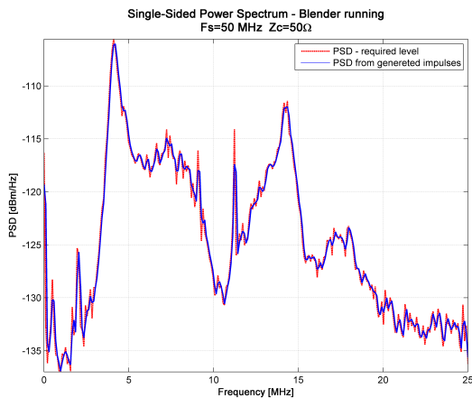
Fig. 14: The required PSD (red line) and PSD from modeled 803 impulses (Blender running).
