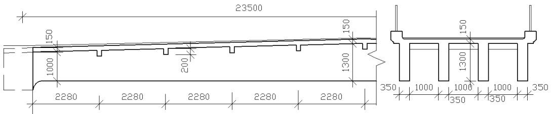
Fig.1: Schematic longitudinal section and cross section in the mid-span of the bridge (dimensions in mm)
