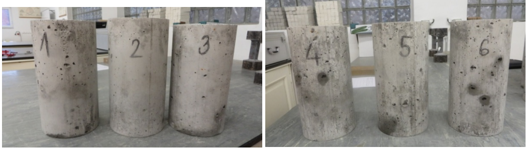
Fig. 1: Six standard cylinders prepared for compression test (1-6) and for evaluation of the static Young modulus (4-6)
