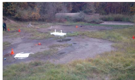
Fig. 18 Spatial distribution of the geophones used in the conducted seismic tests
