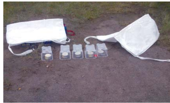
Fig. 17 A view of the used geophones from the companies Austin Detonator Ltd. and Geodyn, Ltd.
