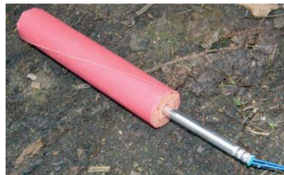
Fig. 8 and 9 Plastic explosive Semtex PI SE M and industrial explosive Perunit E – Ø 28 mm
