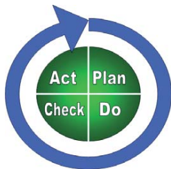
Fig. 5 Deming PDCA cycle as the management guide for continuous product improvement. Its application was later more generalized, and the 'check' stage by Deming renamed 'study' to monitor and investigate results of the 'do' stage and find out what went wrong and how to improve
