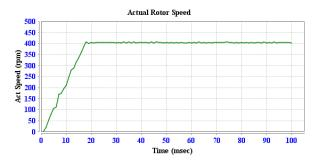
Fig. 16: Low speed operation for reference speed of 400 rpm under no load (Actual rotor speed).
