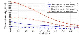
Fig. 1: Modelled results for the VDSL2 transmission rate dependence for NGA network.
