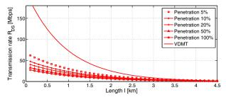
Fig. 2: Model of the VDSL2 length transmission rate dependence for downstream.
