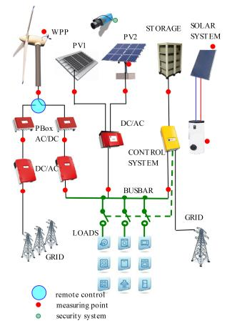
Fig. 1: The block scheme of off-grid power system.
