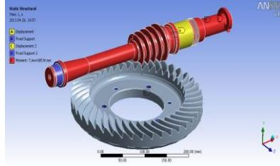
Fig. 4 Setting of charging and marginal conditions
