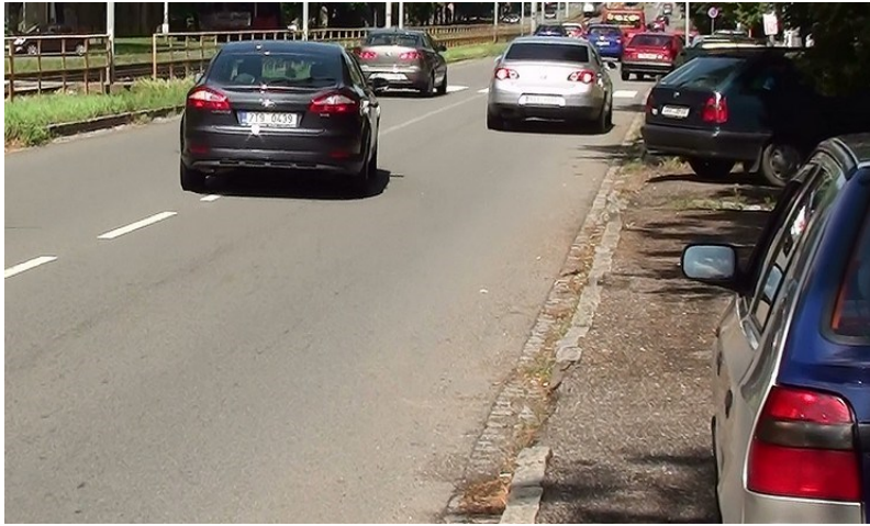
Fig.4. Traffic conflict record. Vehicle decelerating because of parking maneuver is limiting the following vehicle, that had to undertake a severe evasive action [23].
