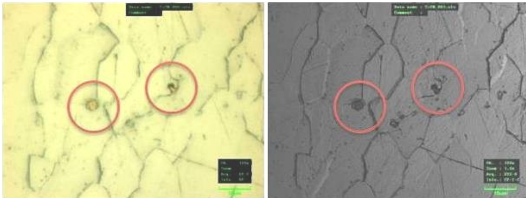
Fig. 1. DC06 ZE50/50 BPO with visible inclusions of TiCN; to the left in a 2D image, to the right as black spots in a 3D image. The images have been magnified 2400 times.
