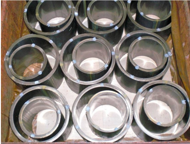
Fig. 2 Stator and rotor packets of position induction sensor.
